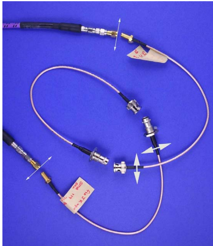
Figure 8 50 Ohm Measurement with SMA Cable Assemblies
