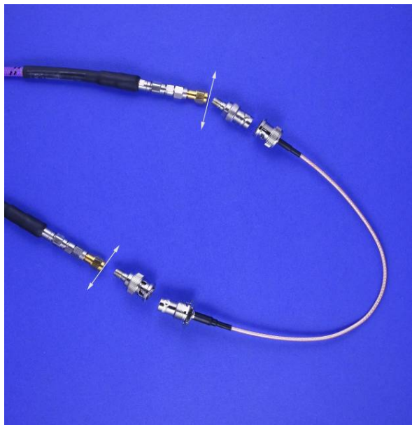
Figure 6 50 Ohm Measurement with Adapter Effects Present
