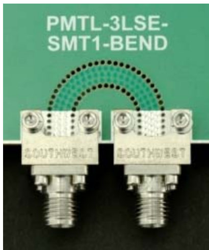
Close up of PMTL transmission line showing the drilled holes in the signal and return paths.
