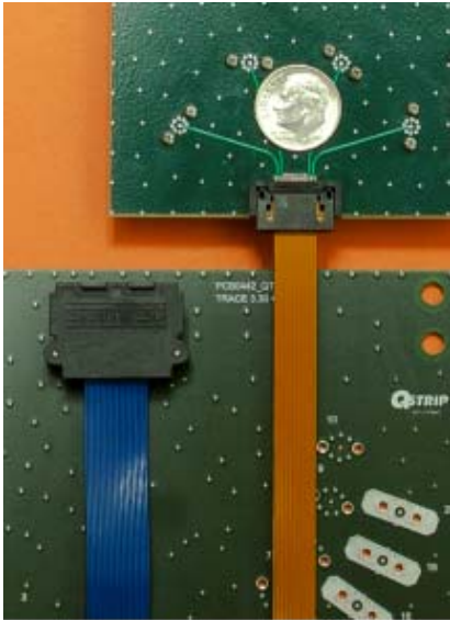
First PMTL product (right) to replace cable assembly (left).
