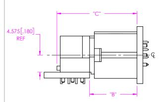
FIG 2 MPTC-V MATED WITH MPSC-RA
