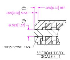
IN PROCESS 3 (PRESS DOWEL PINS)
