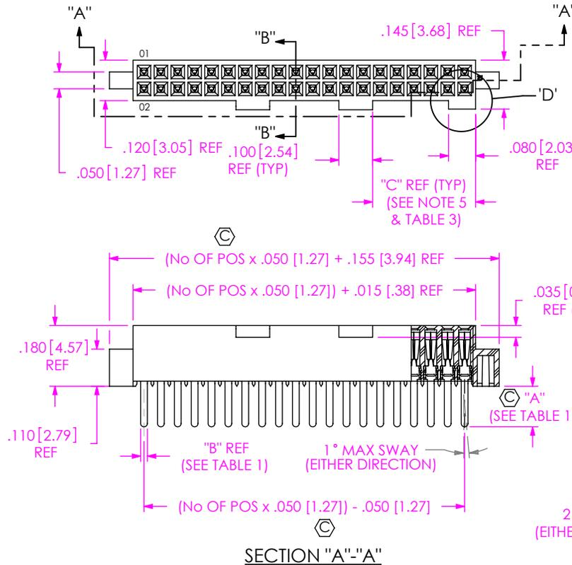
FIG 1 THROUGH HOLE/STRAIGHT MODIFIED (SHOWN: SFML-120-X1-XXX-D)
